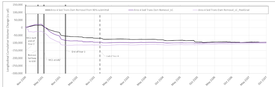
Longitudinal cumulative volume change for the Area 4 TCRA reach using the LC equation with and without a finer pool gradation over the 7-year simulation.
