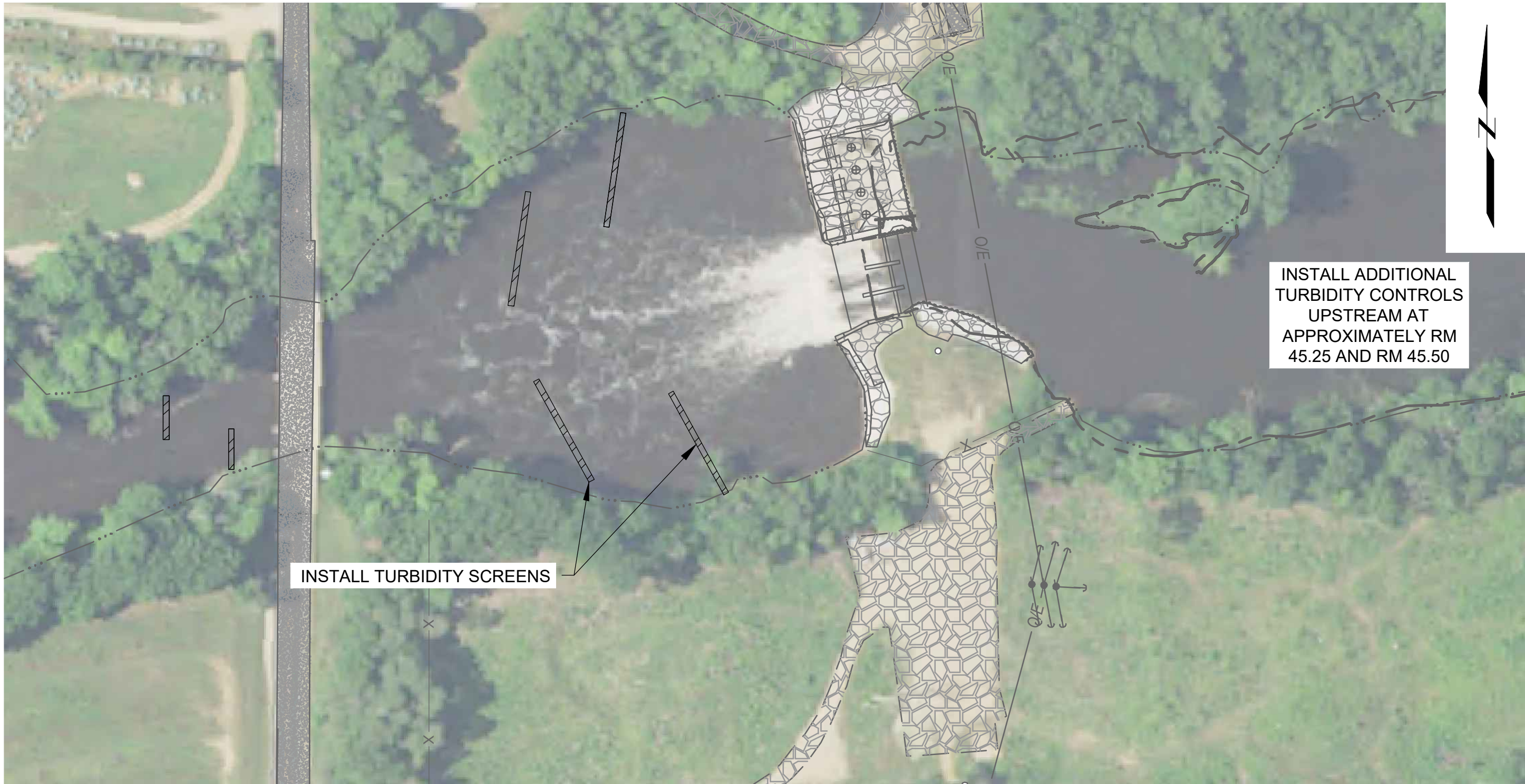
1 STAGE - INSTALL TURBIDITY CONTROLS
