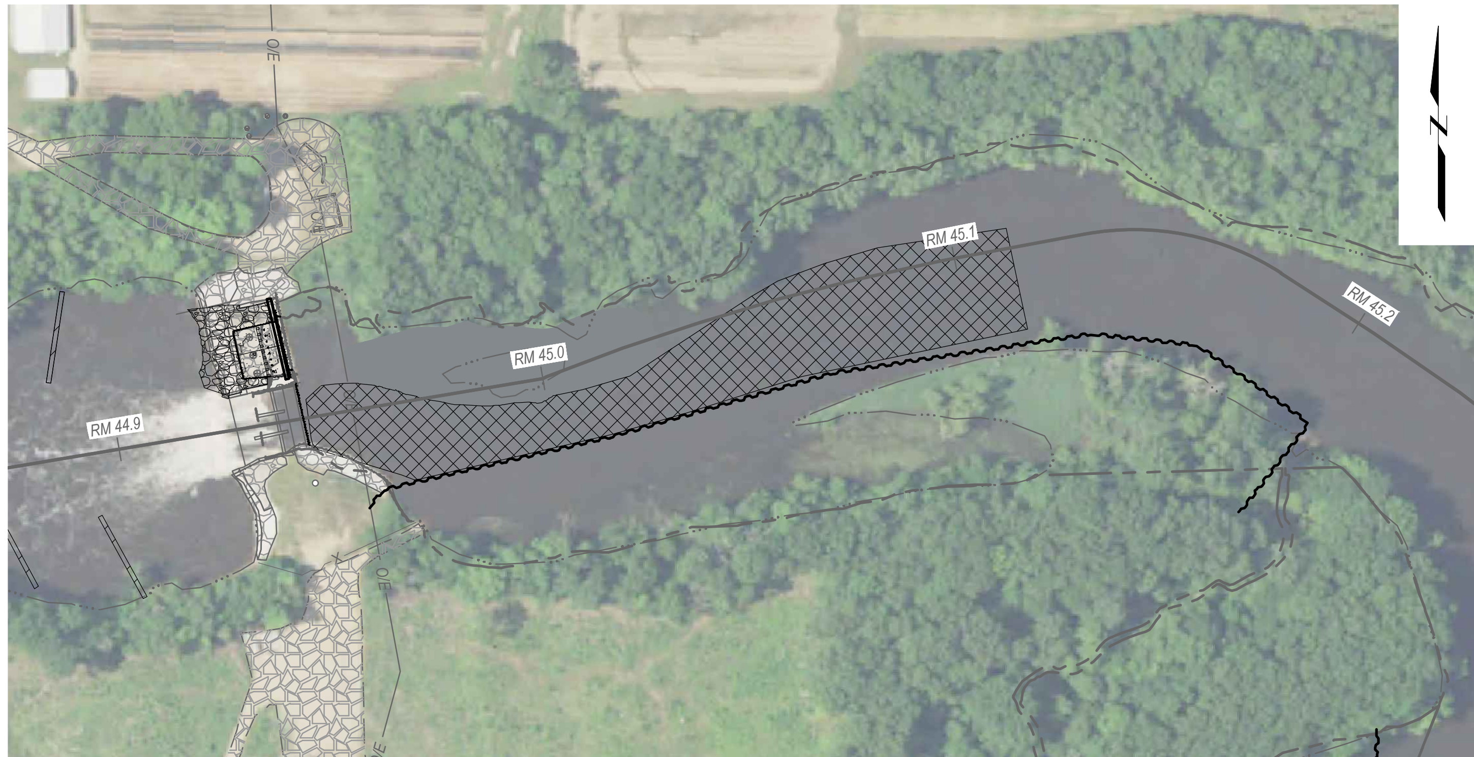
7 - STAGE DREDGE PCB IMPACTED SEDIMENTS IN THE CHANNEL IN LOWER SUBAREA E
