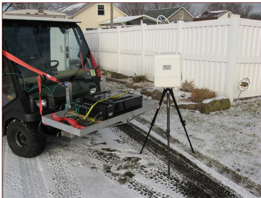
Image 3: Equipment setup on the Kawasaki Mule
