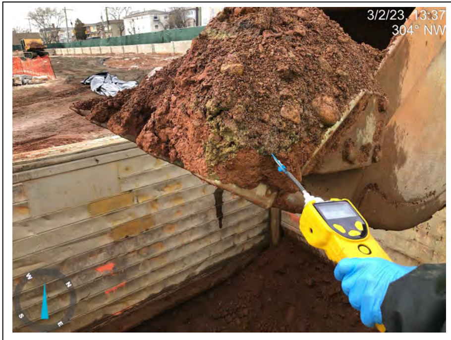
Photograph 32: View of the START V screening a bucket of removed material with a Photoionization Detector (PID) with a VOC sensor at VOC excavation area. The grey material resulted in elevated VOC readings.
