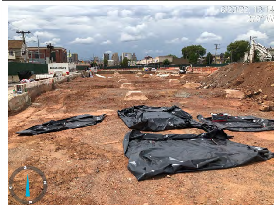
Photograph 11: To conduct a mercury vapor screening of the interior footers of the former buildings, the area and soil around each location was covered with a 12 foot (ft) by (x) 12 ft section of black poly sheeting. To limit the loss of mercury vapors from under the poly sheeting due to the air movement entering under the sheet, four-foot sections of black iron pipe were emplaced around the perimeter of each poly sheet. A total of nine evenly distributed screening points were cut into the poly sheeting: one on top of the footer (top), one on each side of the footer (north, east, south, and west), and one above the soil adjoined to each side of the footer (north soil, east soil, south soil, and west soil). Above is a view of the layout of the screening process.
