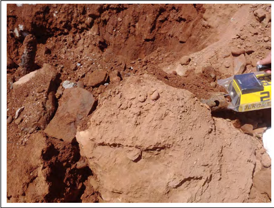
Photograph 36: View of the PRP and their subcontractor conducting mercury vapor readings of a pipe discovered in the footprint of former Building A.
