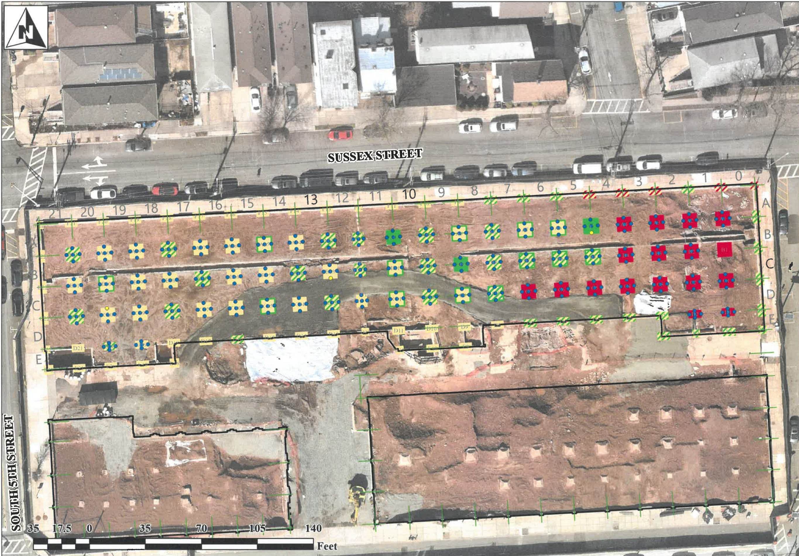
FIGURE 4: VO TOYS FINAL MERCURY SCREENING RESULTS – FOOTER SCREENING BUILDING A
