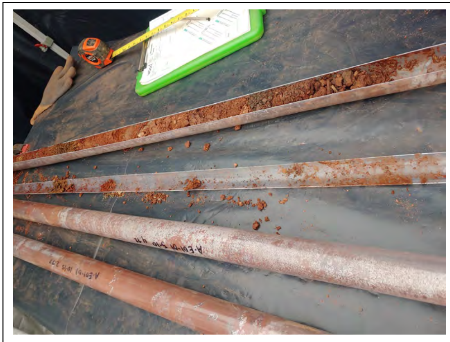
Photograph 21: View of soil core A-E01-01 at 0.0 to 5.0 bgs being processed by the PRP and their subcontractors.
