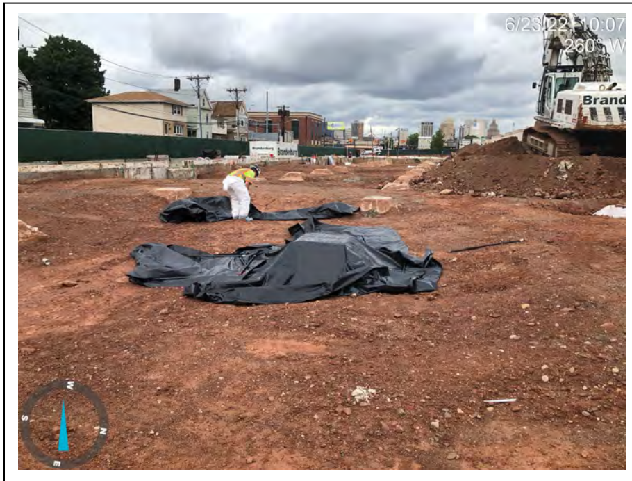
Photograph 10: To conduct a mercury vapor screening of the footers and grids, each area was covered with the black poly sheeting with the perimeter weighted down with iron piping. Each sheet was undisturbed for approximately 10 minutes to heat to above 60 degrees Fahrenheit (°F), which causes mercury to volatilize at a higher rate. START V conducted mercury vapor analyzing with a Lumex 915 +/-M and a Jerome J405. The photo above is a view of START V covering a footer with poly in the Former Building B footprint.
