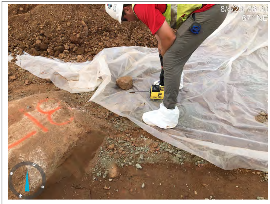
Photograph 40: View of the PRP and their subcontractor conducting soil mercury vapor screening in the footprint of Former Building A. The methodologies for soil mercury vapor screening were modeled after the START V methods described above in Photo 10 and 11.
