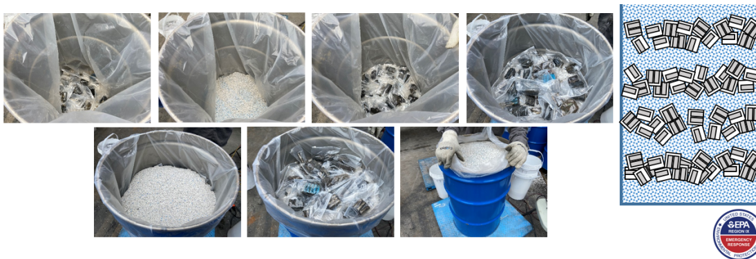
Figure 5: Small lithium-ion batteries can be transported according to DOT Special Permit-16532 in a regular drum with cell block.
