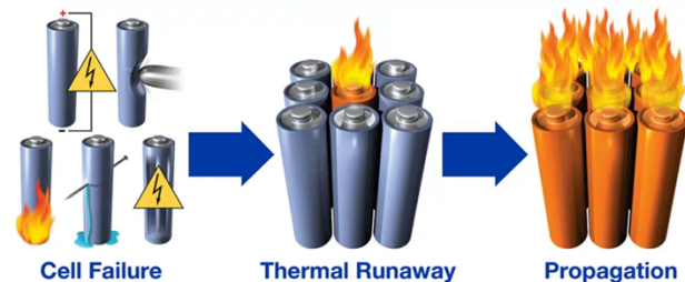
Figure 1: diagram depicting a cascading thermal runaway event
