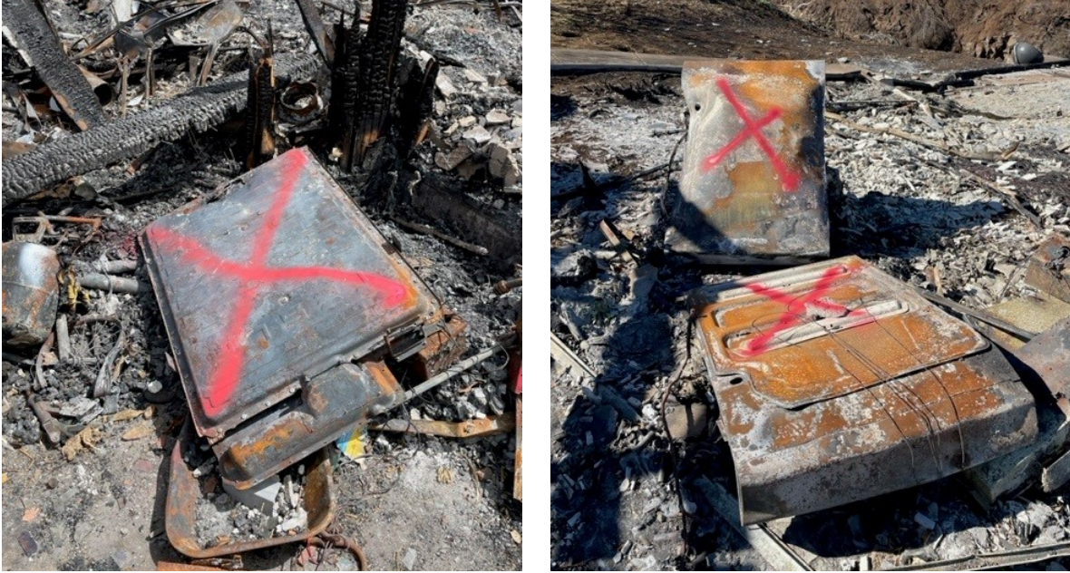
Figure 5: Wildfire damaged Tesla powerwalls
