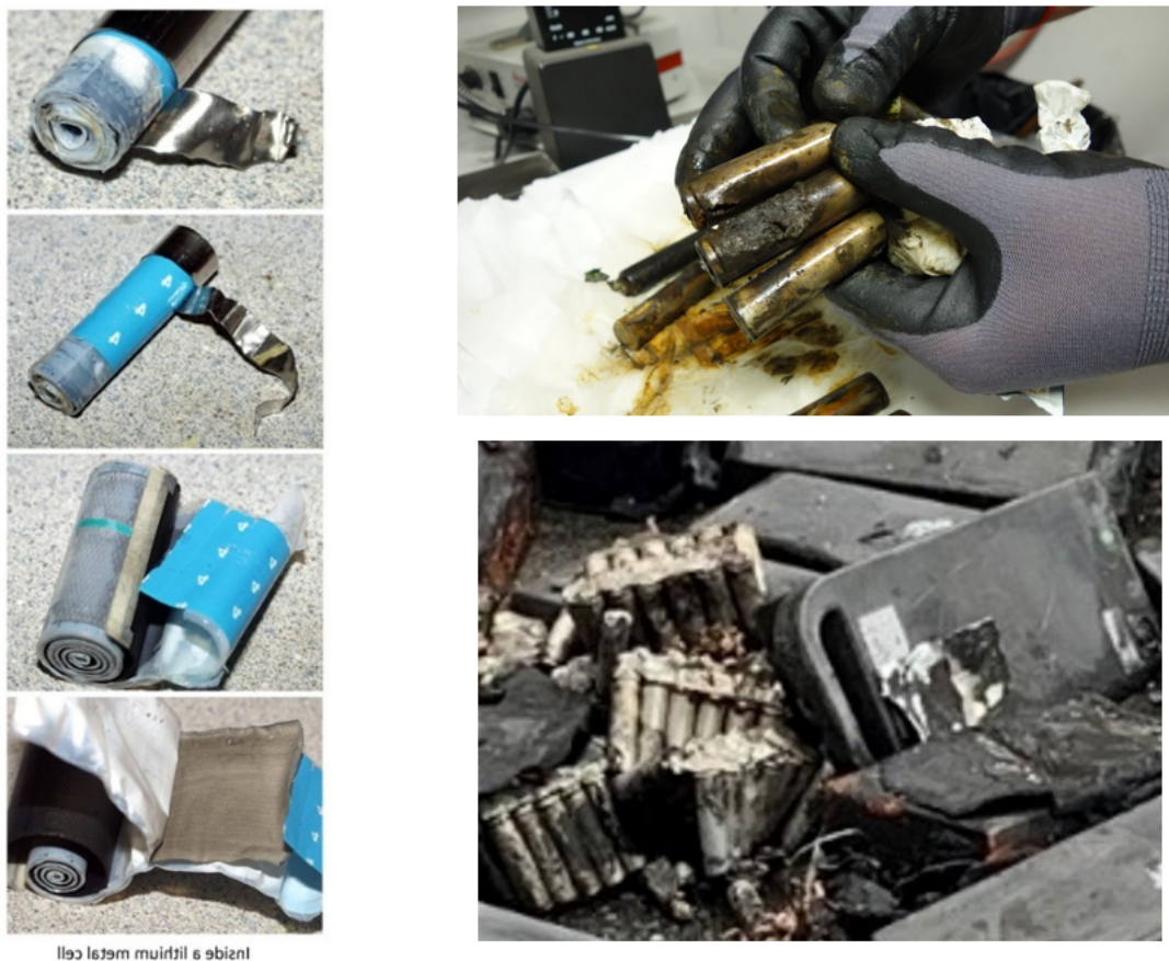
Figure 4: (Left) Lithium-Ion battery cell depicting lithium metal strip rolled up; (Right top) Burned 18650 cells; (right bottom) Fire-damaged pouch-cell batteries
