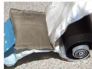
Inside a lithium metal cell
