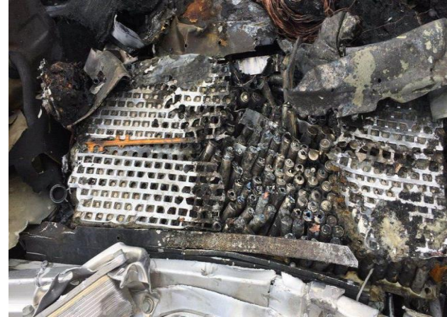
Tesla – Cylindrical Cell Batteries 18650 cell generation
