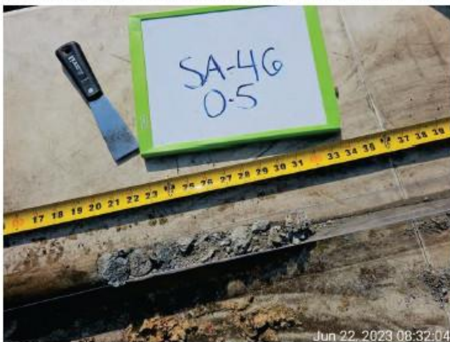
Photograph 16 Orientation: Overview Date: June 22, 2023 Description: Suspect slag drive base from 0–1 foot bgs in the 0–5 feet bgs boring at Sample Location SA-46
