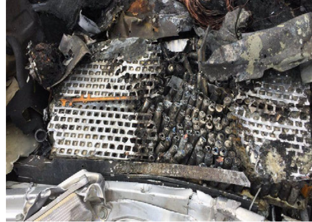
Tesla – Cylindrical Cell Batteries 18650 cell generation
