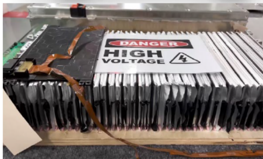
Ford Lightning Battery Pack Pouch Cells
