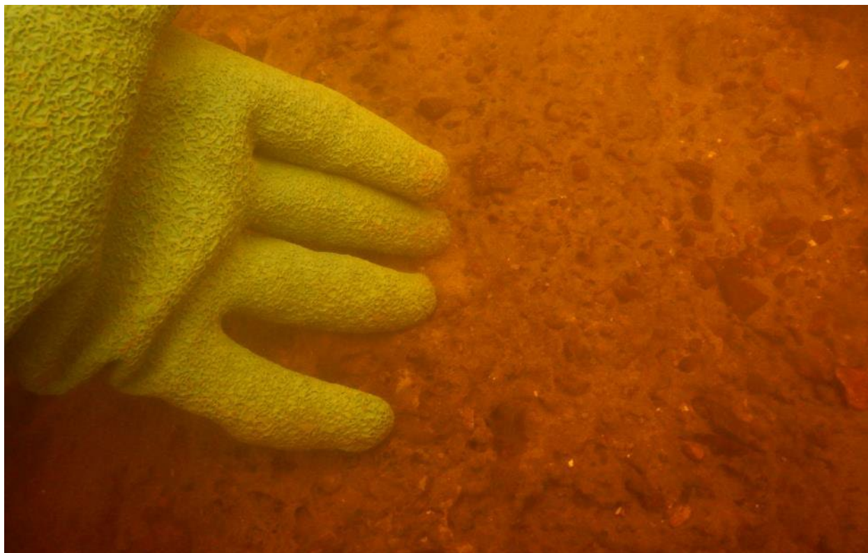
Photo 41. Representative photo showing unsuitable hardpan that is calcified (unable to be excavated) found throughout E3 and E2.
