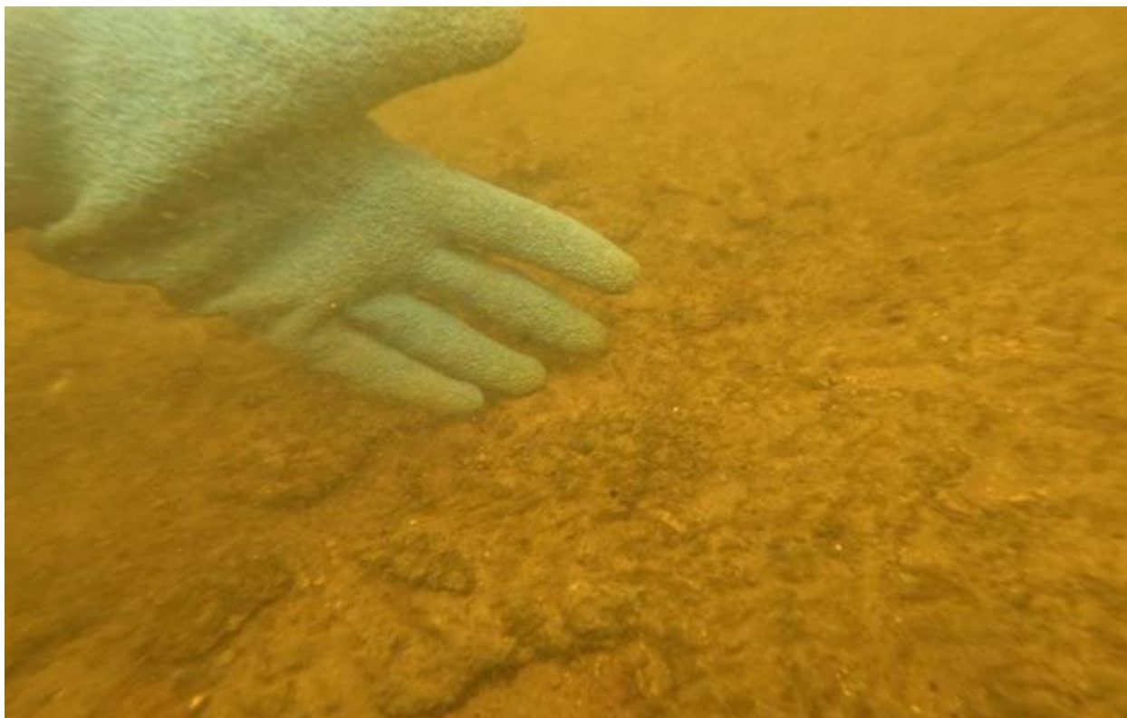
Photo 29. Unsuitable hardpan that is calcified (unable to be excavated) found throughout Sub-Areas C & D.
