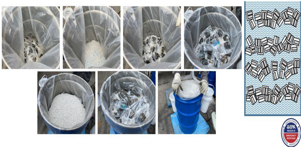
Figure 9: Small lithium-ion batteries can be transported in a regular drum with packing materials.
