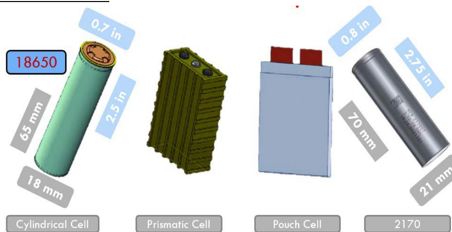
Figure 3: Depiction of lithium-ion battery types.
