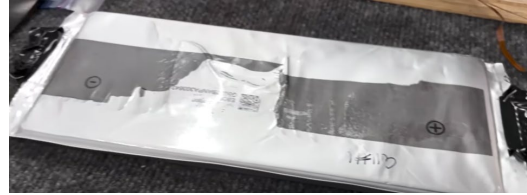
Figure 7: Pouch cell technology has also been identified in use of Ford electric vehicles, such as the Lightning truck model.
