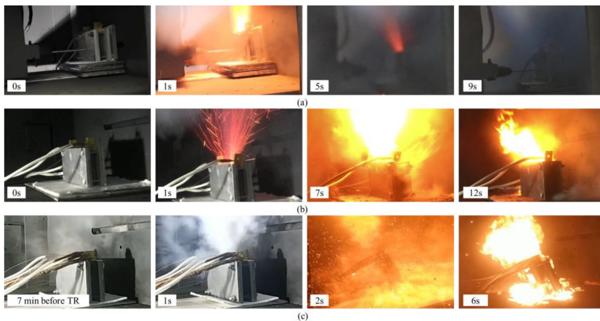
Figure 2: Several views of the stages of lithium-ion batteries in thermal runaway conditions.
