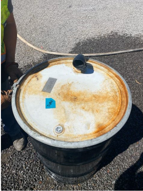
Figure 16: Using 55-gallon drums equipped with a ventilation snorkel can be used to safely store and transport material.
