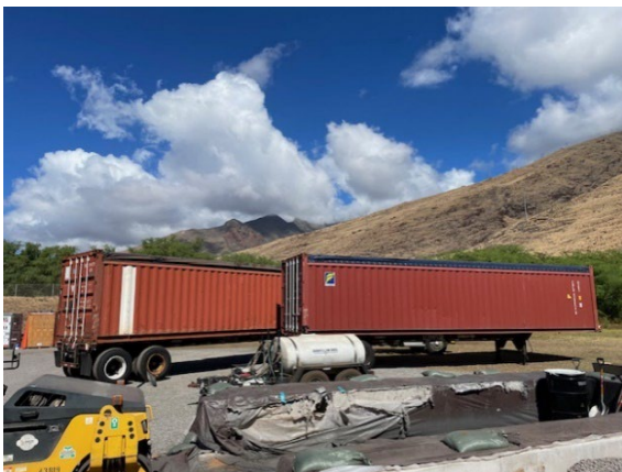
Figure 17: Transport containers that are open top with tarps. These should be placed above-deck when using barge or ship services.
