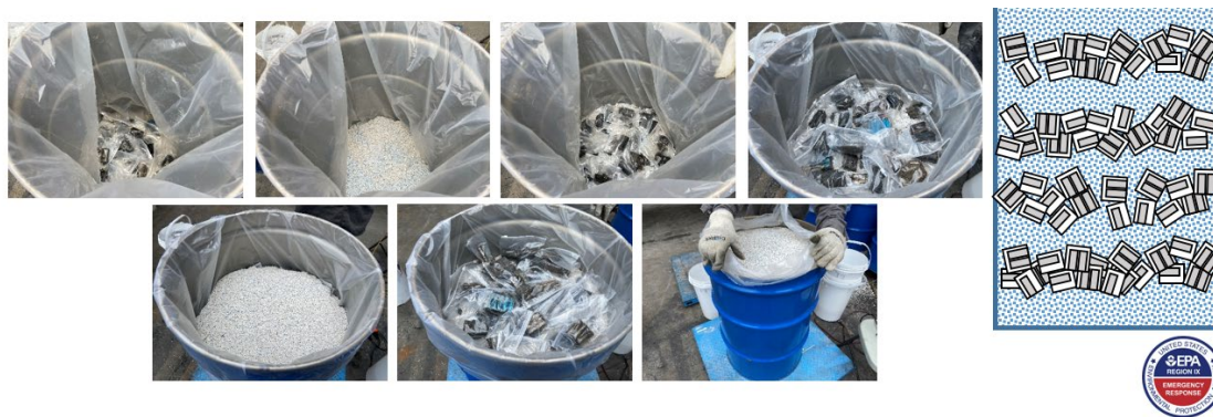
Figure 9: Small lithium-ion batteries can be transported according to Department of Transportation (DOT) Special Permit-16532 in a regular drum with cell block packing materials.
