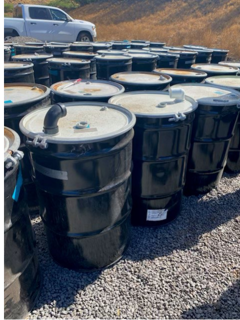
Figure 16: Using 55-gallon drums equipped with a ventilation snorkel can be used to safely store and transport material.
