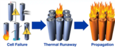
Figure 1: Diagram depicting a cascading thermal runaway event.
