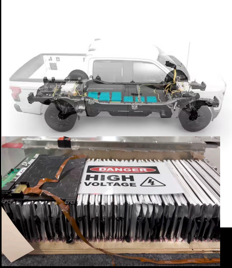
Ford Lightning Battery Pack Pouch Cells
