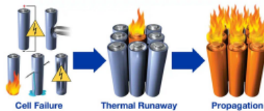
Figure 1: Diagram depicting a cascading thermal runaway event.
