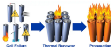
Figure 1: Diagram depicting a cascading thermal runaway event.
